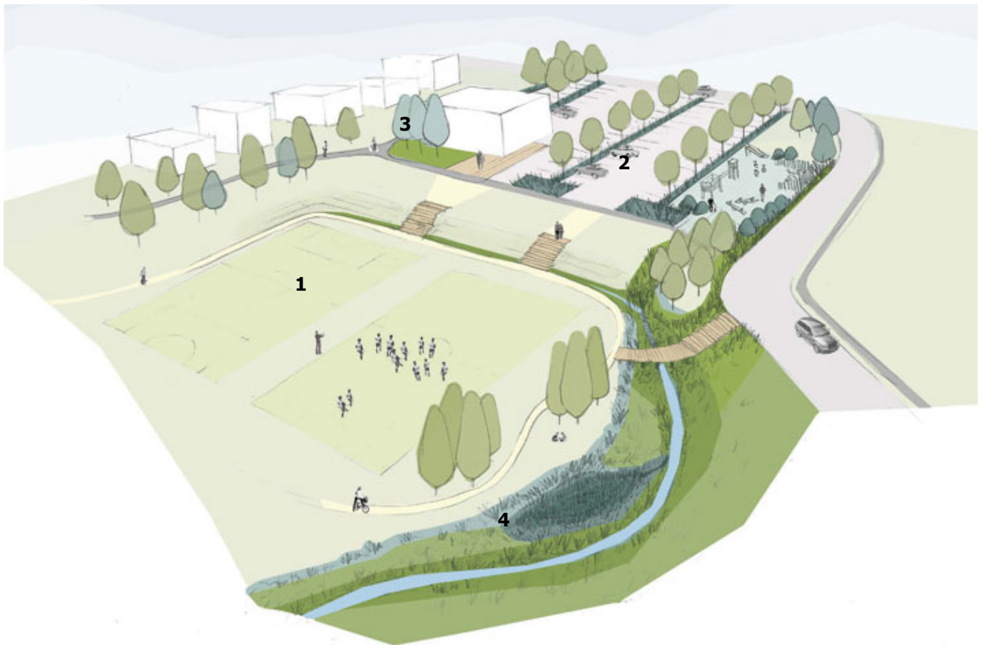
Figure 34: Open spaces can provide enhanced stormwater management functions, while also acting as default storage to detail larger storm events
