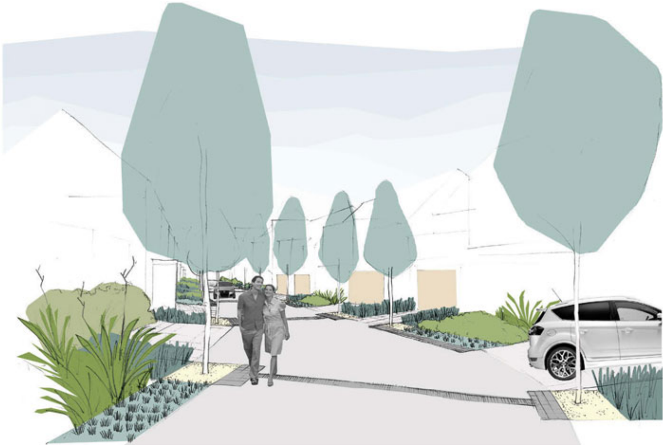
Figure 31: Laneways combine pedestrian and automobile surfaces, providing primary treatment of stormwater and operating as overland flow paths
