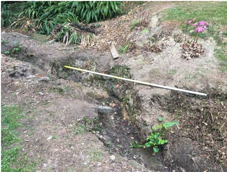
Figure 31: Erosion hotspot exacerbated on private property by poor riparian planting on MIS_MAIN_6.
